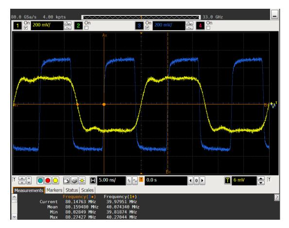
Figure 5.20: Doubled Clock Frequency [73]
