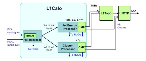
Figure 2.3: L1Calo System Architecture during Run 2 [4]
