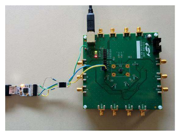
Figure 5.12: Control via External I<sup>2</sup>C Module [63, 54]
