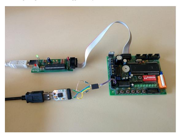
Figure 5.10: I<sup>2</sup>C Communication Test [63, 67, 69]
