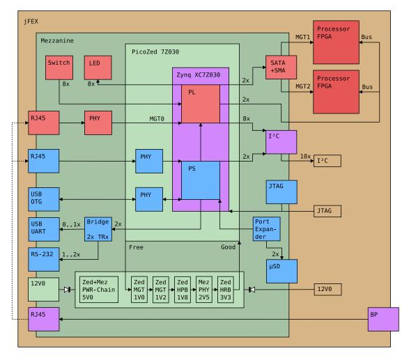
Figure 3.1: Block Diagram of the Mezzanine Card
