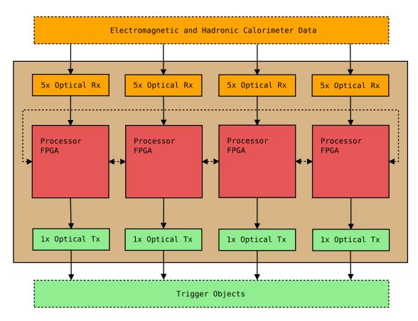
Figure 2.5: Real-Time Data Path of the jFEX
