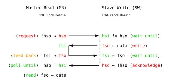
Figure 4.4: Reading From the FPGA
