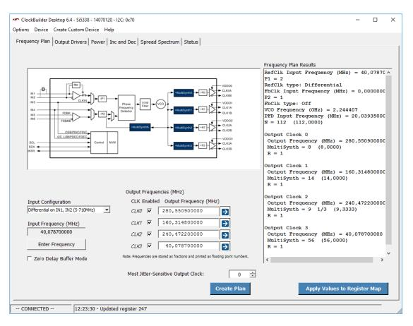
Figure 4.11: Frequency Plan [53]
