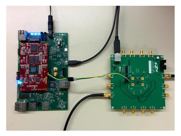
Figure 5.15: Control via Internal I<sup>2</sup>C Module [17, 54]
